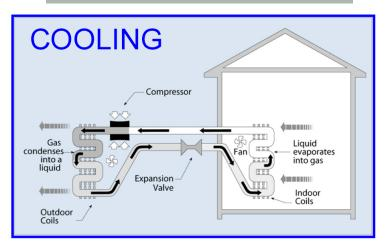
In cooling mode, an air-source heat pump evaporates a refrigerant in the indoor coil; as the liquid evaporates it pulls heat from the air in the house. After the gas is compressed, it passes into the outdoor coil and condenses, releasing heat to the outside air. The pressure changes caused by the compressor and the expansion valve allow the gas to condense at a high temperature outside and evaporate at a lower temperature indoors.
