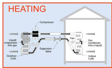
In heating mode, an air-source heat pump evaporates a refrigerant in the outdoor coil; as the liquid evaporates it pulls heat from the outside air. After the gas is compressed, it passes into the indoor coil and condenses, releasing heat to the inside of the house. The pressure changes caused by the compressor and the expansion valve allow the gas to evaporate at a low temperature outside and condense at a higher temperature indoors.
