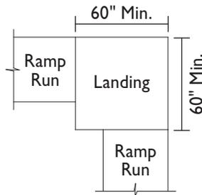
FIG. 106.6.4 RAMP LANDING CHANGE IN DIRECTION – 90° TURN
