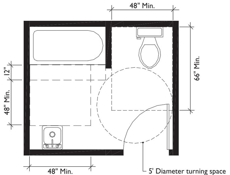
FIG. 301.2 BATHROOM TURNING SPACE AND CLEAR FLOOR SPACE
