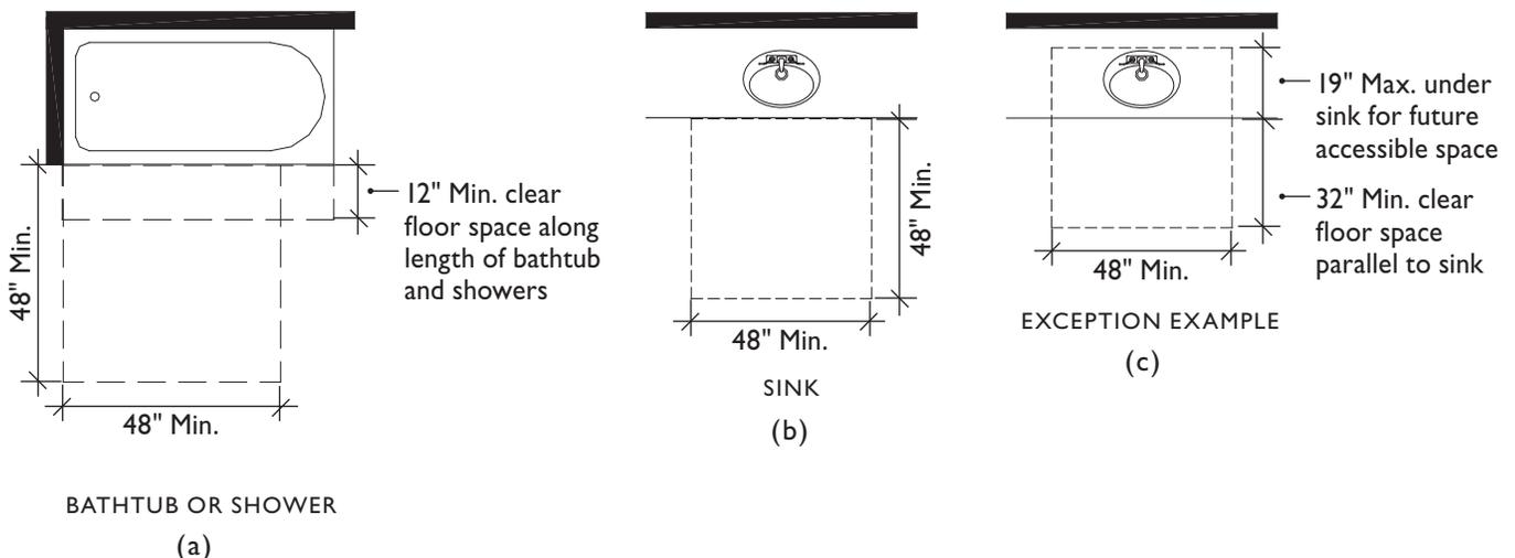
FIG. 301.3 BATHROOM CLEAR FLOOR SPACE
