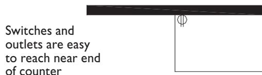
FIG. 601 OPT. 26 SWITCHES AND OUTLETS OVER COUNTERS ON BACK WALL
