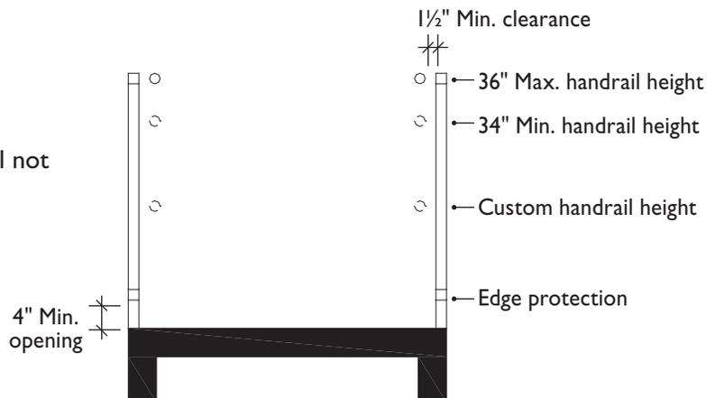
FIG. 106.8 RAMP HANDRAILS
