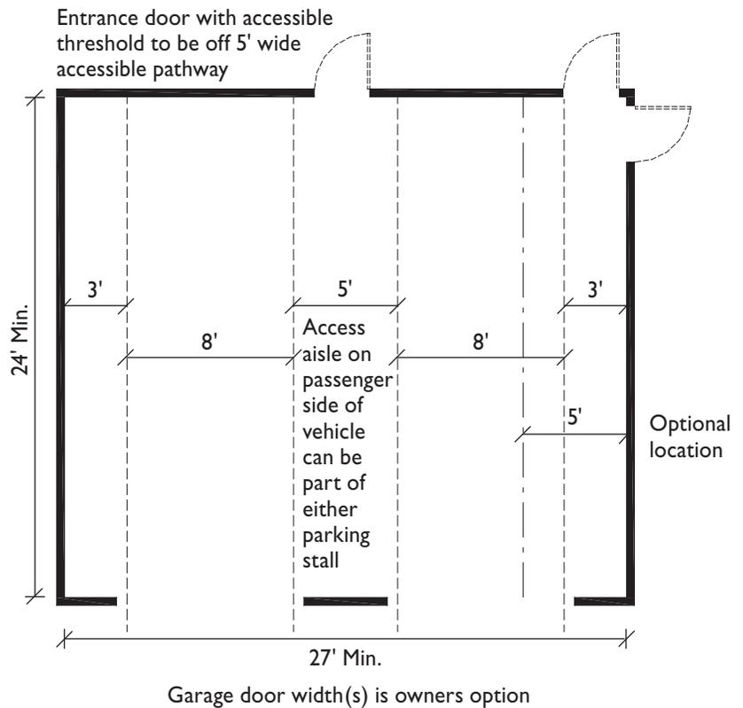
FIG. 103 OPT. 2 MINIMUM MEASUREMENTS TWO STALL GARAGE
