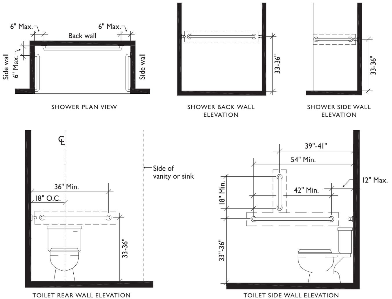
FIG. 301.6 BATHROOM WALL REINFORCEMENT
