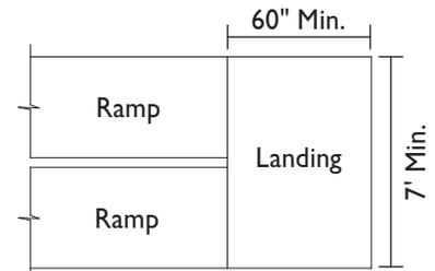
Equal to sum of ramp widths plus space between ramps, if any.
