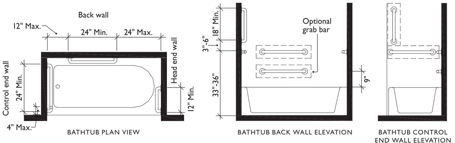
FIG. 301.6 BATHROOM WALL REINFORCEMENT
