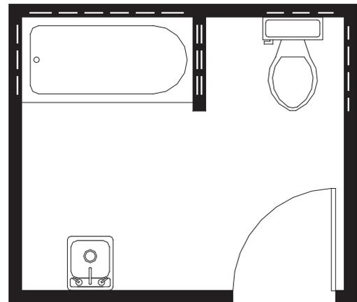
FIG. 301.6 BATHROOM WALL REINFORCEMENT & GRAB BAR LOCATIONS
